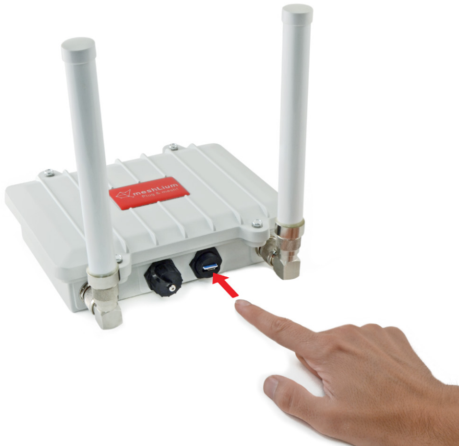
Figure : Inserting a SIM card with care in the External SIM socket
