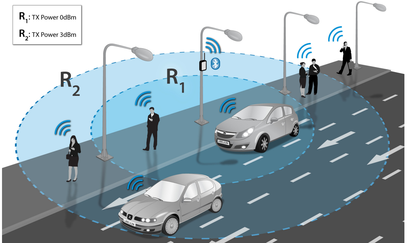
Figure 1.1: Example of TX power levels
