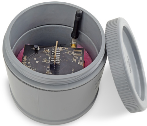
Figure 18: Image of a mote for parking detection introduced in the case
