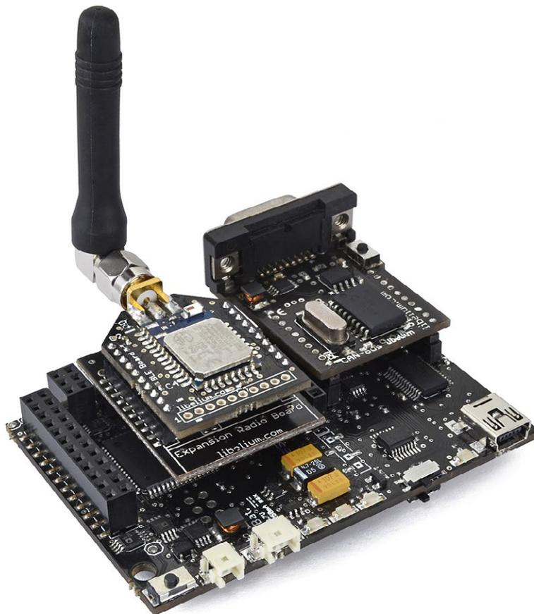
Figure : Wasp mote with CAN Bus module on socket 0 and Bluetooth module on socket 1
