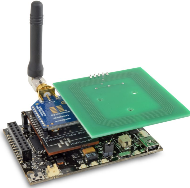
Figure : Waspote with RFID/NFC module on socket 0 (below antenna) and ZigBee radio on socket 1
